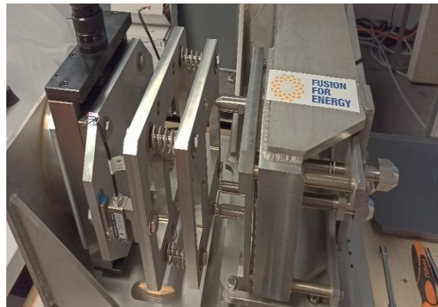
IVVS – Full-scale prototype of the Remote-handing Compatible Connector – it is the high-density electrical/optical connector assembly that services the IVVS Cartridge when installed; it must be connected/disconnected via remote tooling located in the CPRHS
