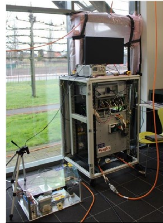
150-m cable communication tests for BiSS module and irradiated ASICs (5 typologies)
