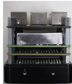
Lab tests on 1-MGy-rated camera sensor (left) and sample image taken after 1MGy \gamma -irradiation (right)
