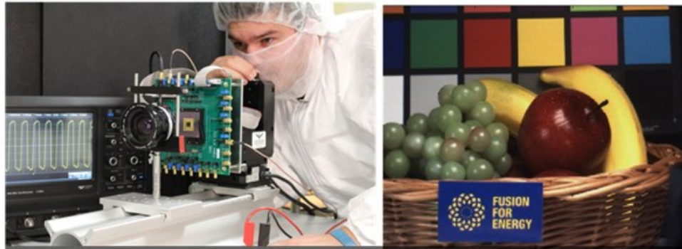
Lab tests on 1-MGy-rated camera sensor (left) and sample image taken after 1MGy \gamma -irradiation (right)
