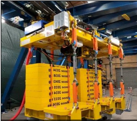
Completion of test campaign on NBRHS crane prototype at Reel premises (France). Extreme offset loading configurations and induced +4 mm rail misalignments trialled
