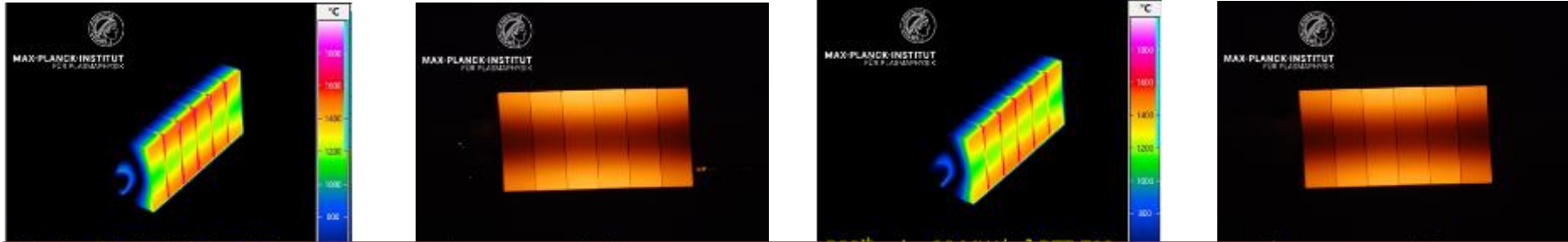
DTT-T02 (4 mm) during the HHF test
