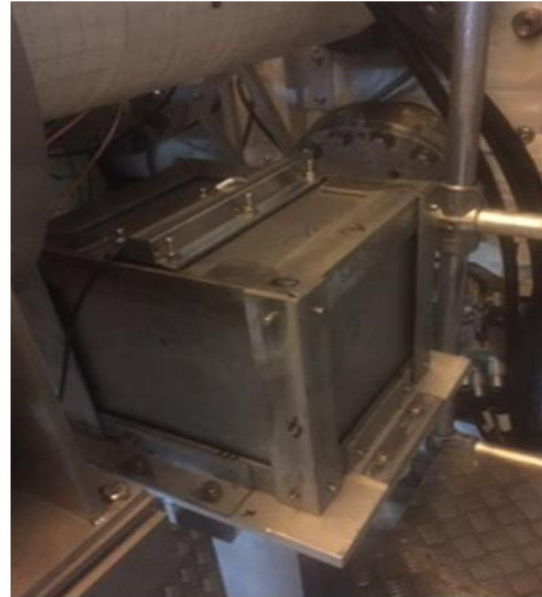
(b) TBM mock-up box
