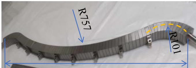
Monoblock component: welded by HIP
