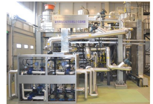
Lead-lithium Loop: 550^{\circ}\text{C} , 2 T, 40 kg/s
