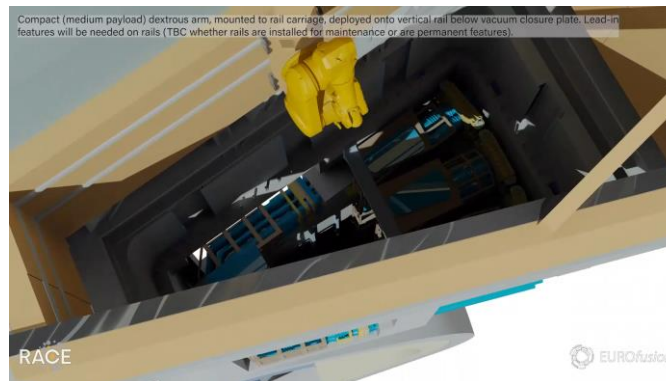
Crane deployed upper port equipment (UKAEA/RACE)
