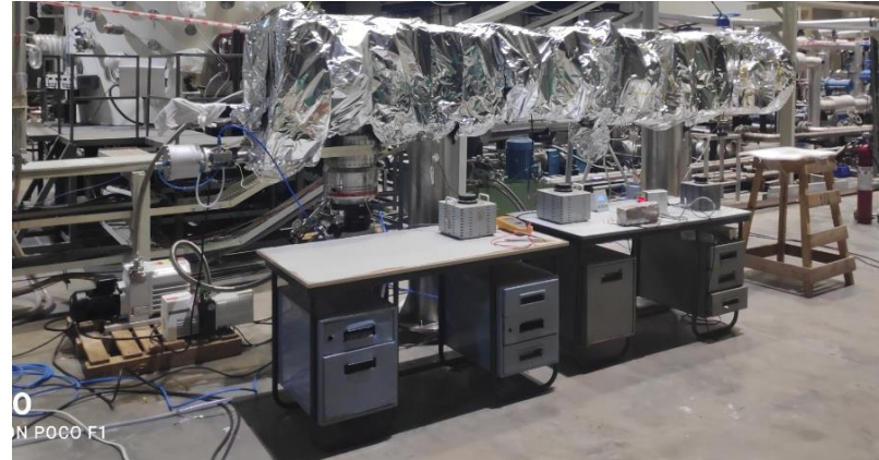
Evacuation of Storage Vacuum Chamber (SVC) with in-situ IVIS) arm with vacuum and baking arrangement
