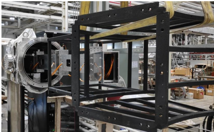
IVIS deployed to maximum reach in atmosphere inside kinematic testing frame
