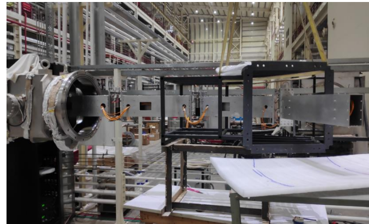
IVIS deployed to maximum reach in atmosphere inside kinematic testing frame
