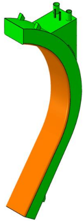
3D FE model of BB segment with no detailed features, e.g. FW cooling channels
