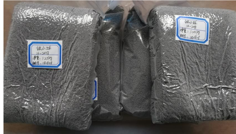
Beryllium pebbles fabricated by REM
