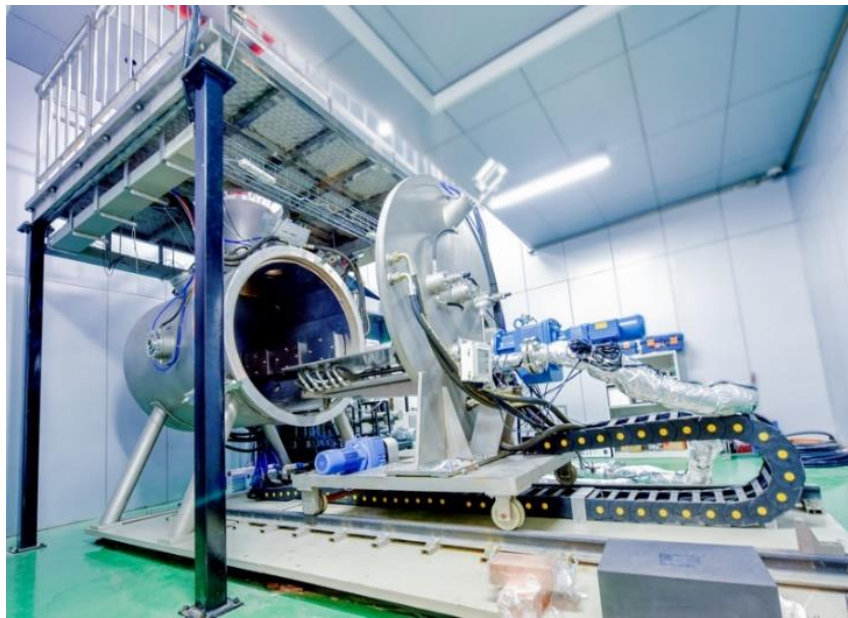
EMS-400 High Heat Flux Testing facility (@SWIP)
