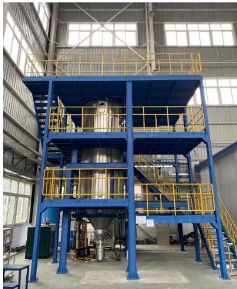
Melt spray method facility @SWIP
