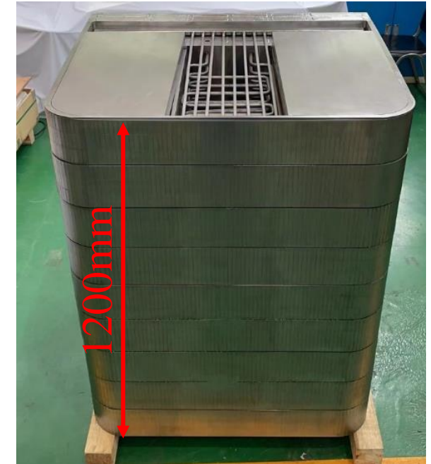
Large size outboard CFETR WCCB blanket module
