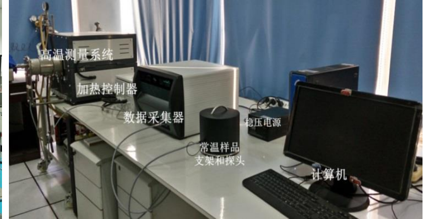
Thermophysical property testing facility
