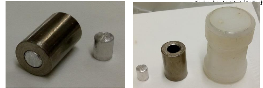
Test rabbit: Nb, Al plugs, Au/Cr/CeO 2 powder filling, PE carrier, F4E FPA-395-02-03
