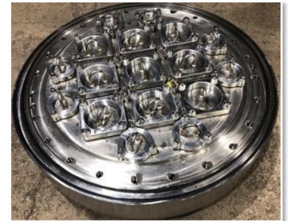
A modified closure plate with 9 additional penetrations was installed in 2022 to expand irradiation capabilities
