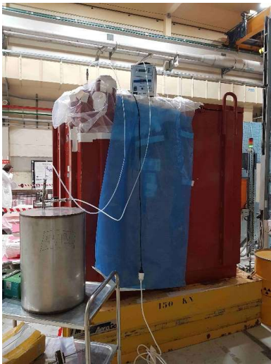
Tritium degassing measurement of a 5m 3 waste package
