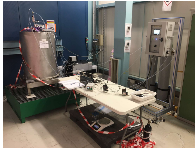
Tritium degassing measurement of 200 L drum
