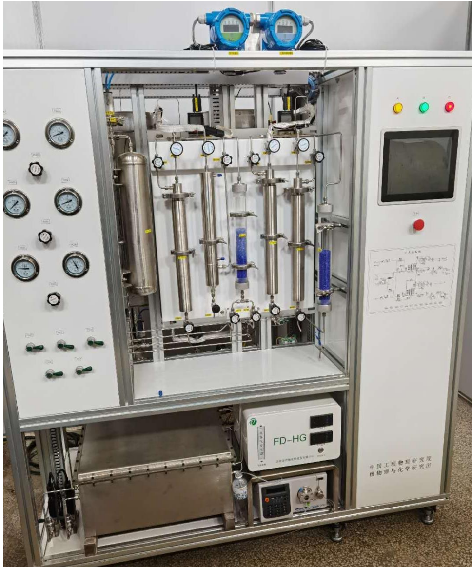
Fig. 4 Picture of the two-stage membrane reactor
