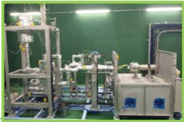
Coolant leakage propagation test
